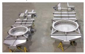
The Bachmann Iso-Spade Guillotine features a single thickness, solid plate blade. Standard configurations of the Bachmann Iso-Spade guillotine and seal arrangements include options for low-leak, tight shut-off and zero-leak, depending on system and customer requirements. It is suitable where "knifing" through medium encrustments is desired, but it, like all flat plate knife gate designs on the market, should be limited to lower temperature applications.
